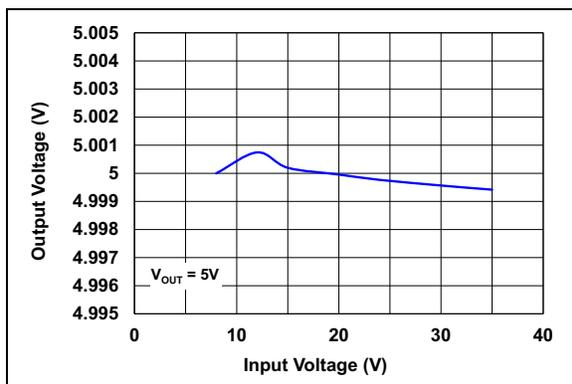
**FIGURE 2-21:** Output Voltage ( $V_{OUT} = 5V$ ) vs. Input Voltage.
