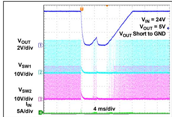
**FIGURE 2-34:**  $V_{OUT}$  Short and Recovery ( $V_{IN} = 24V$ ).
