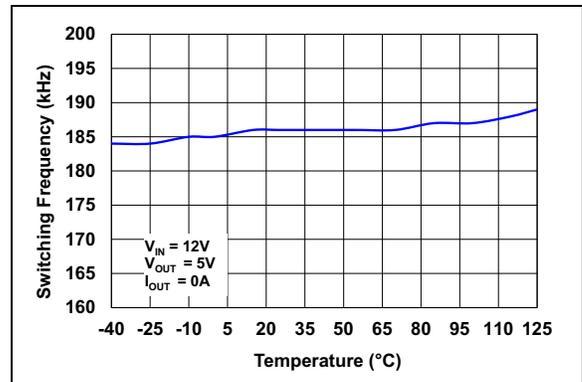
**FIGURE 2-11:** Switching Frequency per Phase vs. Temperature.
