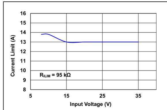
**FIGURE 2-17:** Current Limit per Phase vs. Input Voltage.
