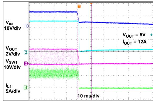
**FIGURE 2-46:** Power-Down with  $V_{IN}$  and 12A Load.
