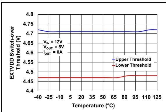
**FIGURE 2-9:** EXT<sub>VDD</sub> Switchover Threshold vs. Temperature.
