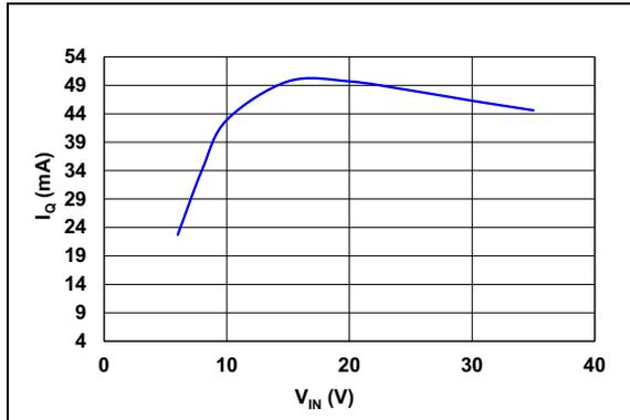
**FIGURE 2-1:**  $V_{IN}$  Operating Current vs. Input Voltage.
