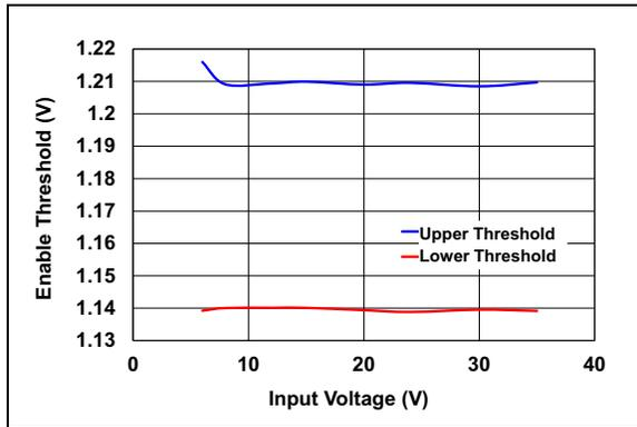
**FIGURE 2-13:** Enable Threshold Voltage vs. Input Voltage.
