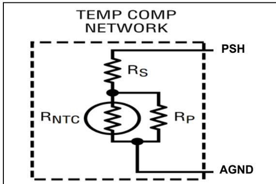
**FIGURE 4-9:** Temperature Compensation Network on the PSH Pin.
