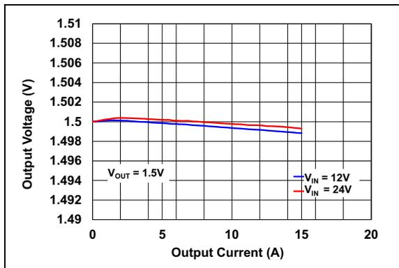
**FIGURE 2-20:** Output Voltage ( $V_{OUT} = 1.5V$ ) vs. Output Current.
