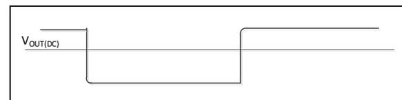
**FIGURE 4-18:**  $V_{OUT}$  Load Transient Error with AVP/DROOP.
