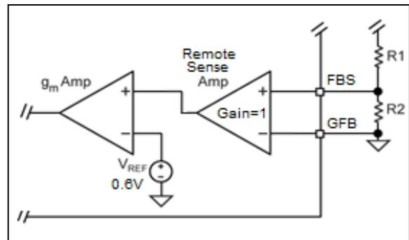
**FIGURE 5-3:** Voltage-Divider Configuration.
