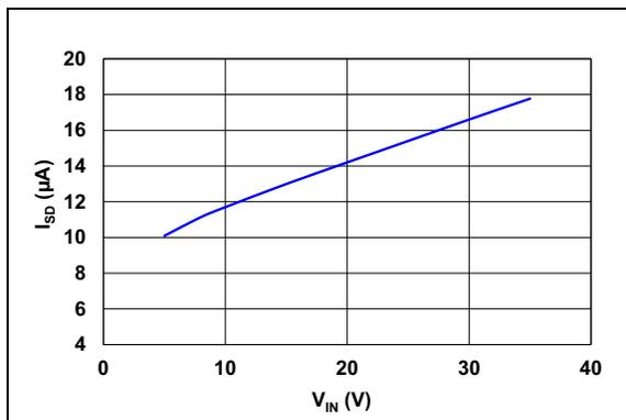
**FIGURE 2-3:**  $V_{IN}$  Shutdown Current vs. Input Voltage.
