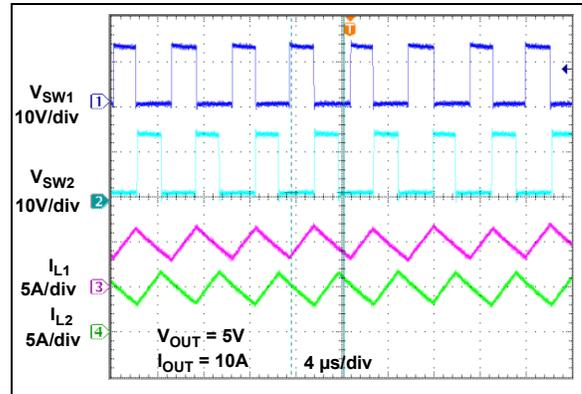
**FIGURE 2-36:** Switching Waveforms Phasing ( $I_{OUT} = 10A$ ).
