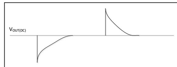
**FIGURE 4-17:**  $V_{OUT}$  Load Transient Error without AVP/DROOP.
