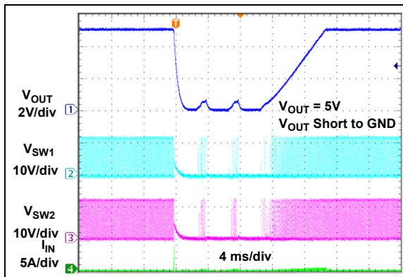
**FIGURE 2-33:**  $V_{OUT}$  Short and Recovery ( $V_{IN} = 12V$ ).
