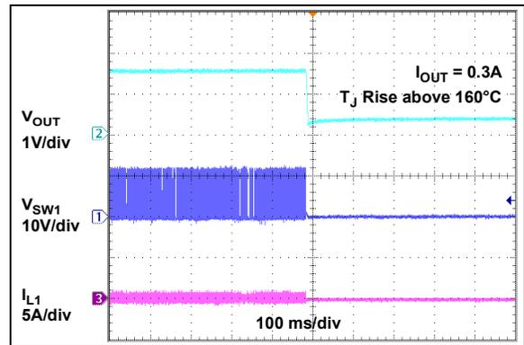
**FIGURE 2-47:** Thermal Shutdown.
