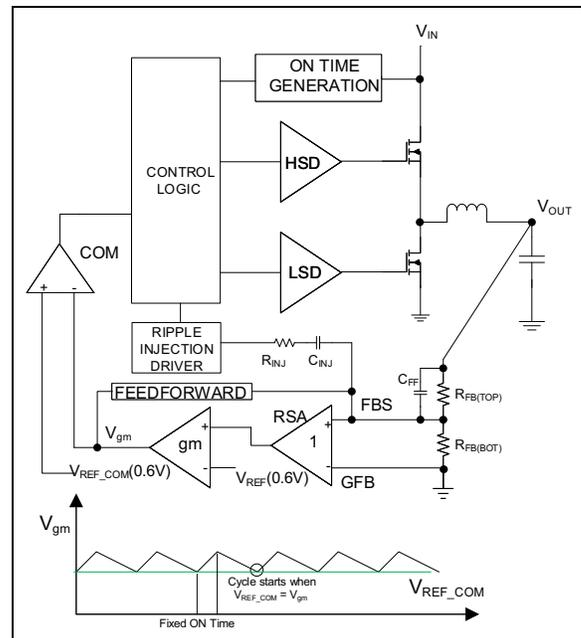
**FIGURE 4-5:** MIC21LV33 Ripple Injection at FBS Node.
