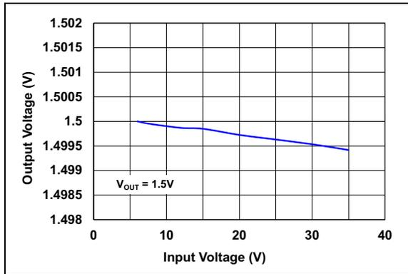
**FIGURE 2-19:** Output Voltage ( $V_{OUT} = 1.5V$ ) vs. Input Voltage.
