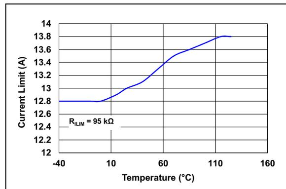
**FIGURE 2-18:** Current Limit per Phase vs. Temperature.
