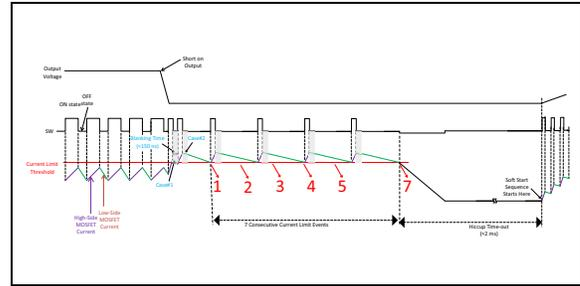
**FIGURE 4-11:** MIC21LV33 Current-Limit Threshold Relationship to Output Current.
