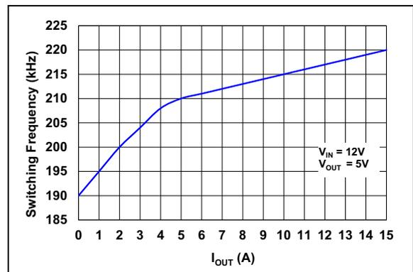
**FIGURE 2-12:** Switching Frequency per Phase vs. Output Current.
