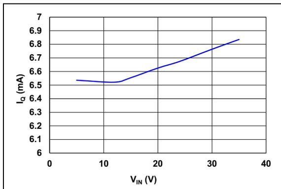
**FIGURE 2-2:**  $V_{IN}$  Quiescent Current vs. Input Voltage.
