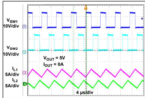
**FIGURE 2-35:** Switching Waveforms Phasing ( $I_{OUT} = 0A$ ).
