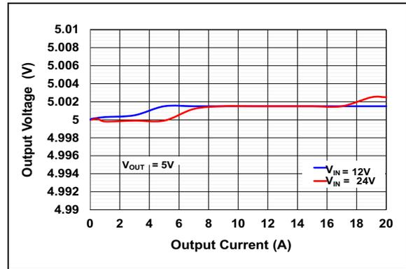
**FIGURE 2-22:** Output Voltage ( $V_{OUT} = 5V$ ) vs. Output Current.
