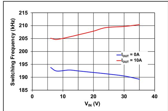
**FIGURE 2-10:** Switching Frequency per Phase vs. Input Voltage.
