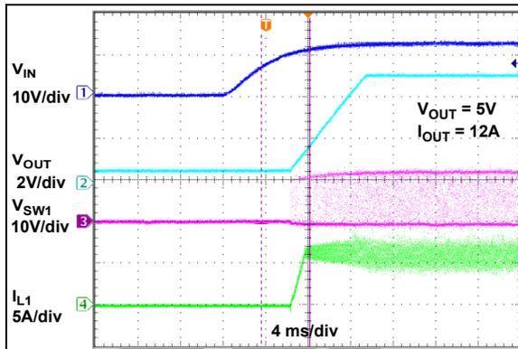
**FIGURE 2-45:** Power-up with  $V_{IN}$  and 12A Load.
