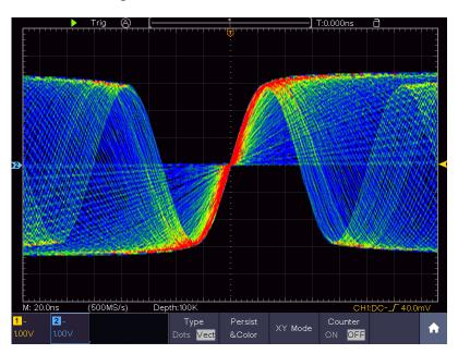
Figure 4-6 The color temperature function is on
