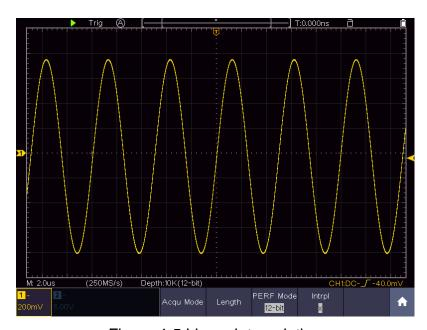
Figure 4-5 Linear interpolation
