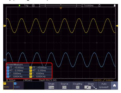
Figure 4-18 Automatic measurement
