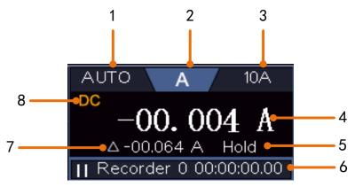
Figure 5-3 Multimeter Information Window
