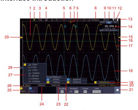
Figure 3-4 Illustrative Drawing of Display Interfaces
