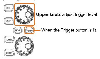
Figure 3-12 Trigger Control Zone
