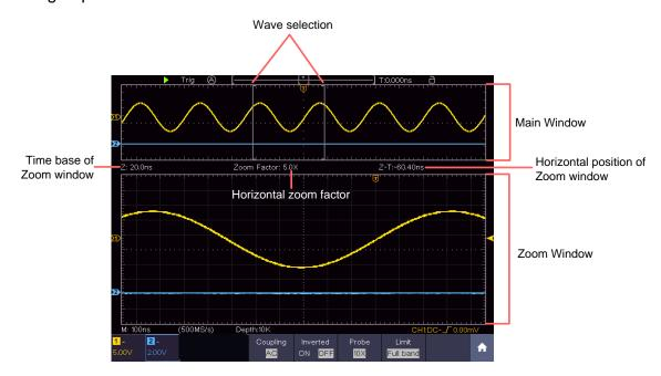
Figure 4-2 Waveform Horizontal Zooming Mode
