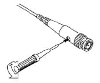
Figure 3-7 Adjust Probe
