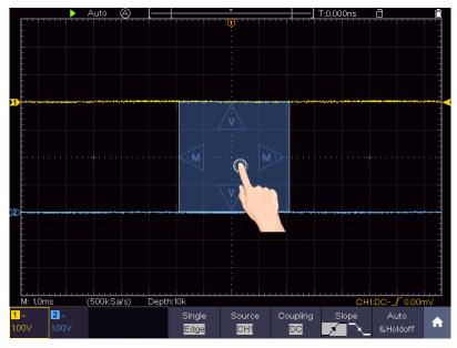
When the **M** and **V** icons appear, in the full screen, swipe left/right to change the time base, swipe up/down to change the voltage division of the selected channel.
