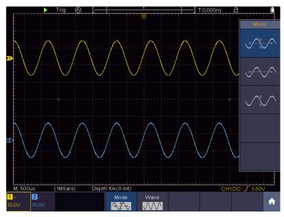
Figure 4-23 Autoscale Horizontal-Vertical multi-period waveforms
