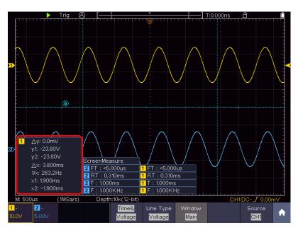
Figure 4-21 Time&Voltage Cursor Measurement
