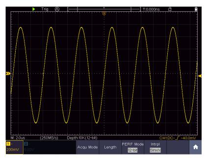
Figure 4-4 Sine(x)/x interpolation
