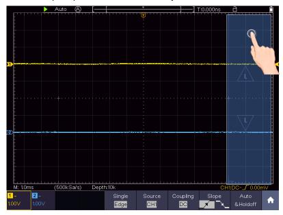
When the  $\bf L$  icon appears, in the full screen, swipe up/down to control the trigger level of the source in the trigger menu.
