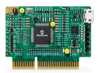
dsPIC33CH512MP506 Digital Power Plug-In Module (Part # MA330049)
