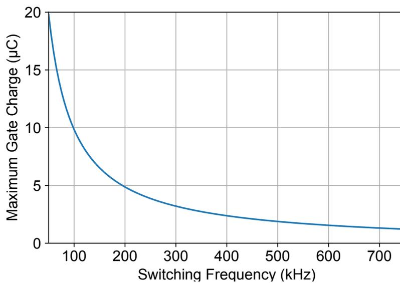
**Figure 2.17. Maximum Gate Charge vs. Switching Frequency**
