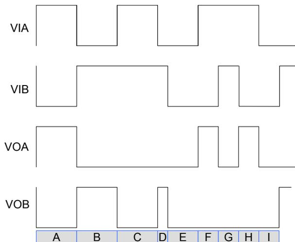
Figure 2.19. Input and Output Waveforms for Si8273x Drivers
