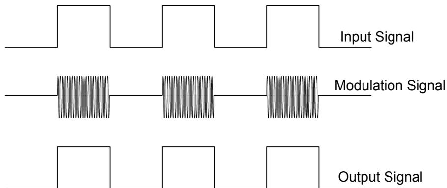
Figure 2.6. Modulation Scheme
