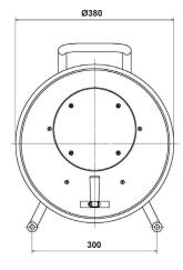
**Cable Capacity Guide:** Reel Bend Radius = 120mm
