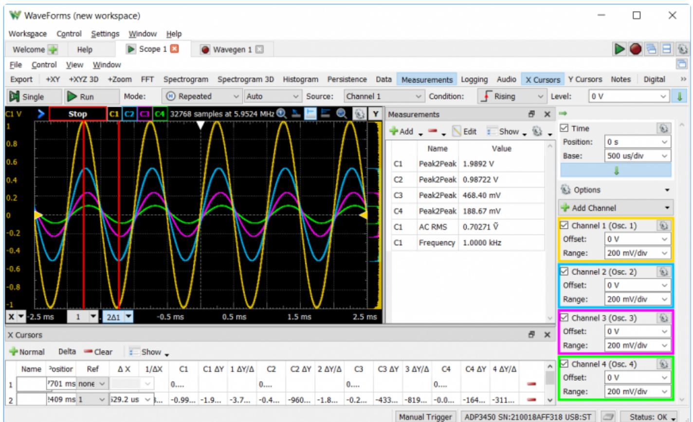
The Analog Discovery Pro (ADP3450/ADP3250) can be used with WaveForms' Oscilloscope instrument to capture analog data via the 4 analog input ("Scope") channels using BNC probes.
