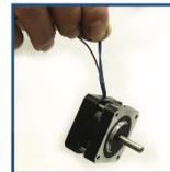
**Do not** hold motor by lead wires.
