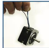
**Do not** hold motor by lead wires.
