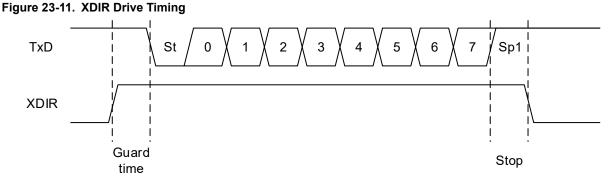
Writing RS485[1] to '1' enables the RS-485 mode, which automatically sets the TXD pin to output one clock cycle before starting transmission and sets it back to input when the transmission is complete.
