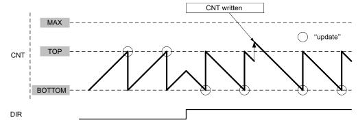
It is possible to change the counter value in the Counter (TCAn.CNT) register when the counter is running. The write access to TCAn.CNT register has higher priority than count, clear or reload, and will be immediate. The direction of the counter can also be changed during normal operation by writing to the Direction (DIR) bit in the Control E (TCAn.CTRLE) register.
