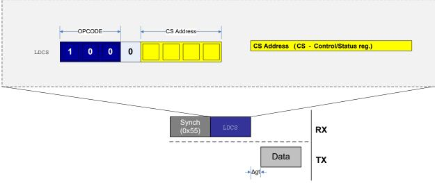
Figure 30-11 shows a typical example of LDCS data transmission. A data byte from the LDCS is transmitted from the UPDI after the guard time is completed.
