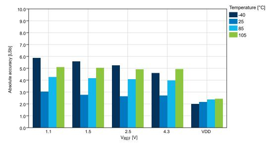
Figure 33-45. Absolute Accuracy vs. V<sub>REF</sub> (V<sub>DD</sub> = 5.0V, f<sub>ADC</sub> = 115 ksps), REFSEL = Internal Reference
