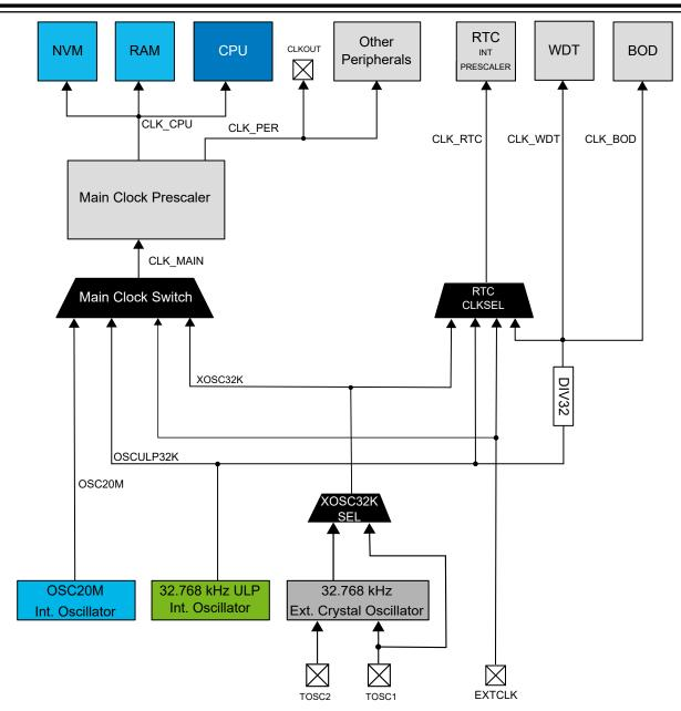
The clock system consists of the main clock and other asynchronous clocks:
