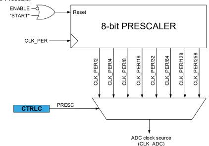
The ADC requires an input clock frequency between 50 kHz and 1.5 MHz for maximum resolution. If a lower resolution than ten bits is selected, the input clock frequency to the ADC can be higher than 1.5 MHz to get a higher sample rate.
