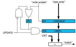
Both the TCAn.CMPn and TCAn.CMPnBUF registers are available as I/O registers. This allows the initialization and bypassing of the buffer register and the double-buffering function.
