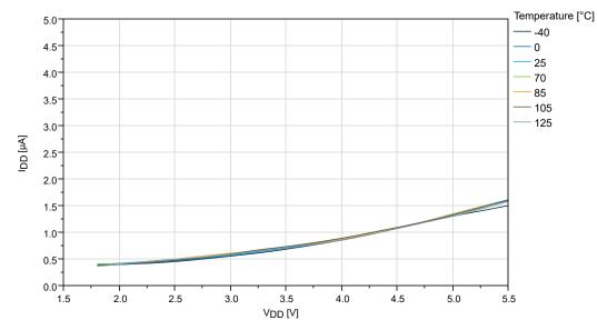
Figure 33-39. BOD Current vs.  $V_{DD}$  (Sampled BOD at 125 Hz)
