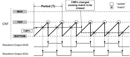
The figure below shows how the waveform can be inverted by changing CMPn during run-time.
