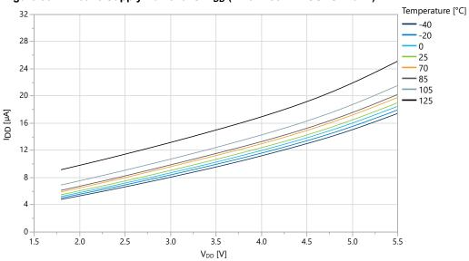
Figure 33-7. Active Supply Current vs. V<sub>DD</sub> (f = 32.768 kHz OSCULP32K)
