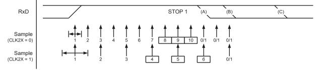
A new high-to-low transition indicating the Start bit of a new frame can come right after the last of the bits used for majority voting. For Normal-Speed mode, the first low-level sample can be at the point marked (A) in the figure above. For Double-Speed mode, the first low level must be delayed to point (B), being the first sample after the majority vote samples. Point (C) marks a Stop bit of full length at the nominal baud rate.
