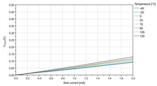
Figure 33-24. I/O Pin Output Voltage vs. Sink Current (V<sub>DD</sub> = 3.0V)
