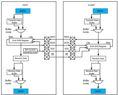
The SPI is built around an 8-bit shift register that will shift data out and in at the same time. The Transmit Data register and the Receive Data register are not physical registers but are mapped to other registers when written or
