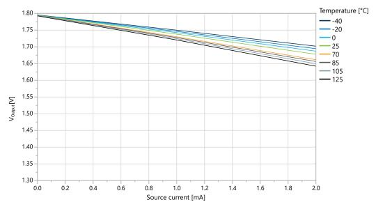
Figure 33-27. I/O Pin Output Voltage vs. Source Current (V<sub>DD</sub> = 1.8V)
