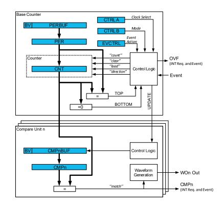
The Counter (TCAn.CNT) register, Period and Compare (TCAn.PER and TCAn.CMPn) registers, and their corresponding buffer registers (TCAn.PERBUF and TCAn.CMPnBUF) are 16-bit registers. All buffer registers have a Buffer Valid (BV) flag that indicates when the buffer contains a new value.
