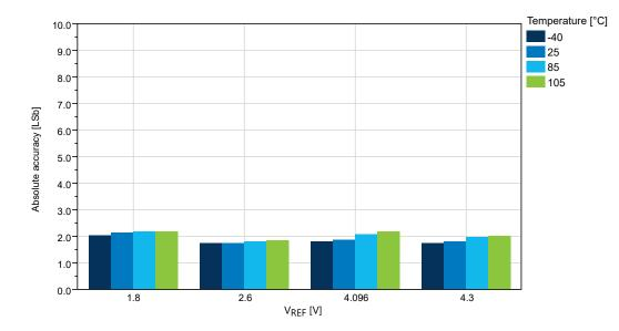
Figure 33-55. Absolute Accuracy vs. V<sub>REF</sub> (V<sub>DD</sub> = 5.0V, f<sub>ADC</sub> = 115 ksps, REFSEL = External Reference)
