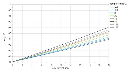
Figure 33-25. I/O Pin Output Voltage vs. Sink Current (V<sub>DD</sub> = 5.0V)
