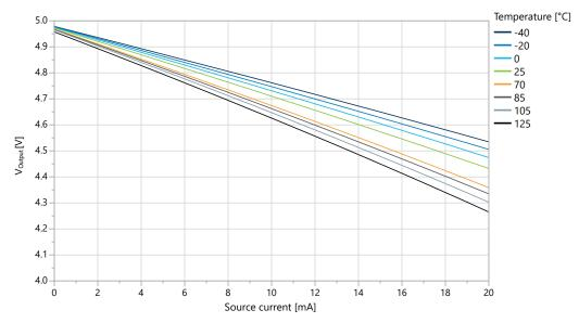
Figure 33-29. I/O Pin Output Voltage vs. Source Current (V<sub>DD</sub> = 5.0V)
