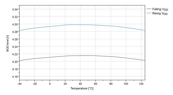
Figure 33-43. BOD Threshold vs. Temperature (BODLEVEL7)
