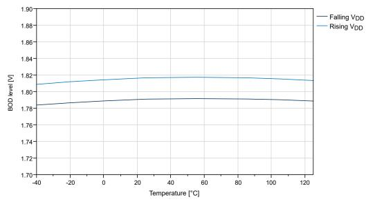
Figure 33-42. BOD Threshold vs. Temperature (BODLEVEL2)
