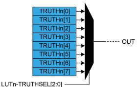
The truth table inputs (LUTn-TRUTHSEL[2:0]) are configured by writing the Input Source Selection bit fields in the
