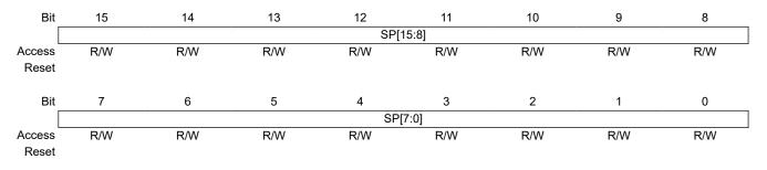
**Bits 15:8 – SP[15:8]** Stack Pointer High Byte These bits hold the MSB of the 16-bit register.
