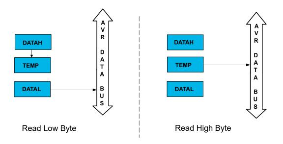
For a 16-bit read operation, the low byte register (e.g., DATAL) of the 16-bit register must be read before the high byte register (e.g., DATAH). When the low byte register is read, the high byte register of the 16-bit register is copied into the temporary (TEMP) register in the same clock cycle, as shown on the left side of the figure above. Reading the high byte register will result in a read from TEMP instead of the high byte register, as shown on the right side of the same figure.
