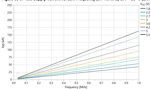
Figure 33-9. Idle Supply Current vs. Low Frequency (0.1-1.0 MHz) at T = 25 °C (EXTCLK)
