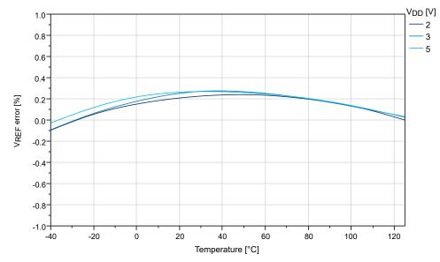
Figure 33-35. Internal 1.1V Reference vs. Temperature
