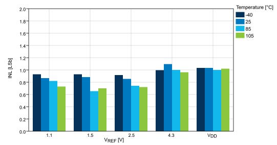
Figure 33-51. INL vs. V<sub>REF</sub> (V<sub>DD</sub> = 5.0V, f<sub>ADC</sub> = 115 ksps), REFSEL = Internal Reference
