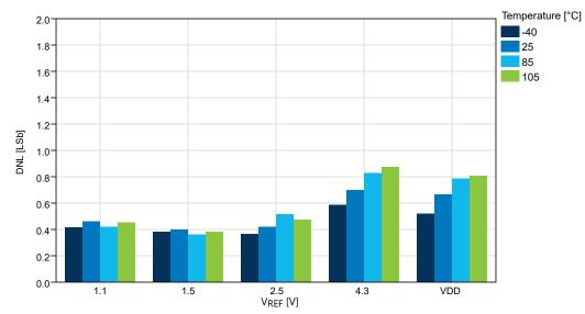
Figure 33-47. DNL vs. V<sub>REF</sub> (V<sub>DD</sub> = 5.0V, f<sub>ADC</sub> = 115 ksps), REFSEL = Internal Reference
