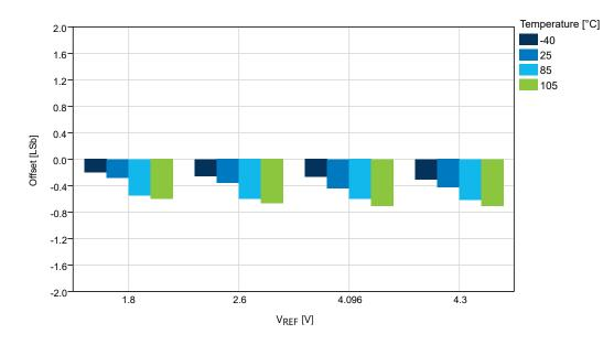
Figure 33-63. Offset vs. V<sub>REF</sub> (V<sub>DD</sub> = 5.0V, f<sub>ADC</sub> = 115 ksps, REFSEL = External Reference)
