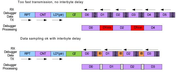
In Figure 30-17, GT denotes the Guard Time insertion, SB is for Stop Bit and IB is the inserted interbyte delay. The rest of the frames are data and instructions.
