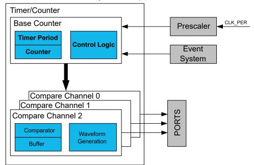
Figure 20-1. 16-bit Timer/Counter and Closely Related Peripherals
