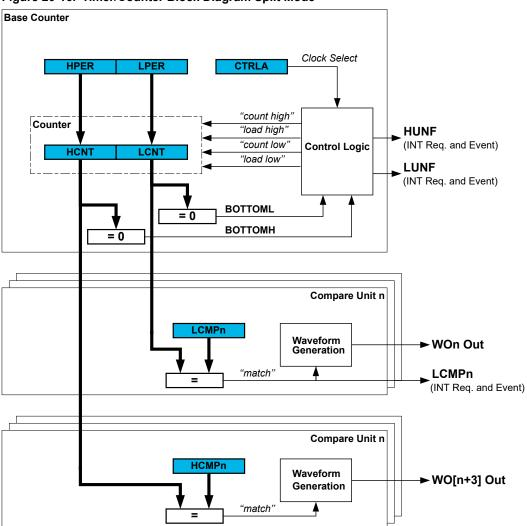
Figure 20-16. Timer/Counter Block Diagram Split Mode
