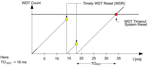
Normal mode is enabled as long as the WINDOW bit field in the Control A (WDT.CTRLA) register is 0x0.
