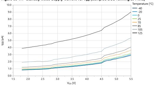
Figure 33-17. Standby Mode Supply Current vs. V<sub>DD</sub> (Sampled BOD running at 1 kHz)
