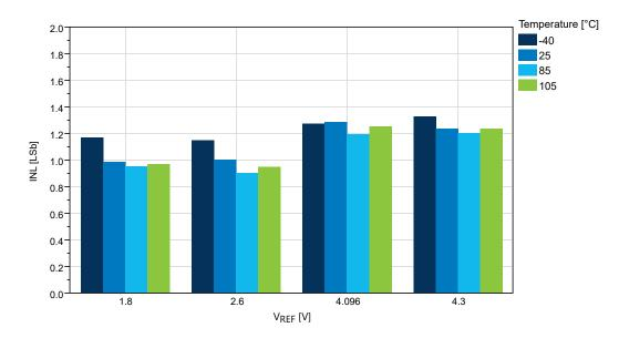
Figure 33-61. INL vs. V<sub>REF</sub> (V<sub>DD</sub> = 5.0V, f<sub>ADC</sub> = 115 ksps, REFSEL = External Reference)
