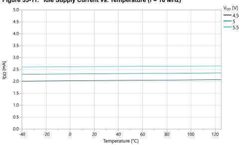
Figure 33-11. Idle Supply Current vs. Temperature (f = 16 MHz)
