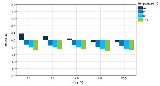
Figure 33-53. Offset Error vs. V<sub>REF</sub> (V<sub>DD</sub> = 5.0V, f<sub>ADC</sub> = 115 ksps), REFSEL = Internal Reference
