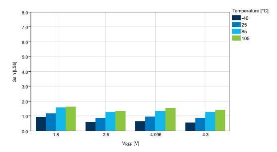
Figure 33-59. Gain vs. V<sub>REF</sub> (V<sub>DD</sub> = 5.0V, f<sub>ADC</sub> = 115 ksps, REFSEL = External Reference)
