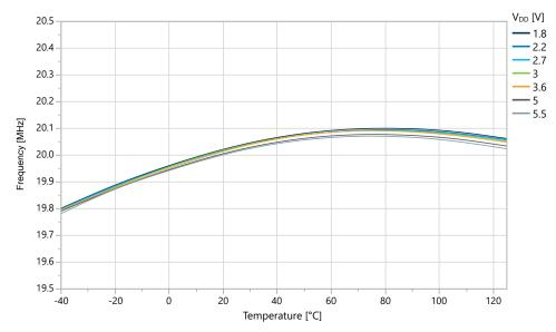
Figure 33-71. OSC20M Internal Oscillator: Frequency vs. Temperature
