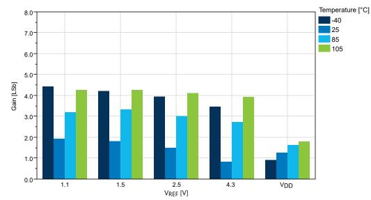
Figure 33-49. Gain Error vs. V<sub>REF</sub> (V<sub>DD</sub> = 5.0V, f<sub>ADC</sub> = 115 ksps), REFSEL = Internal Reference
