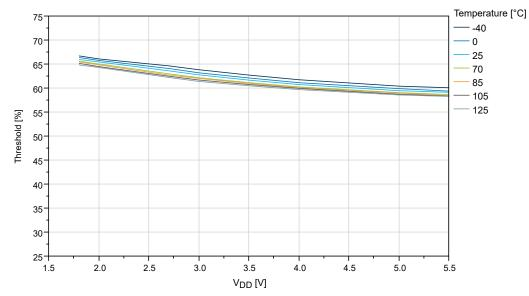
Figure 33-21. I/O Pin Input Threshold Voltage vs. V<sub>DD</sub> (V<sub>IH</sub>)
