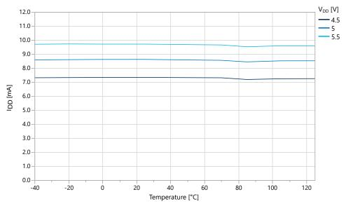
Figure 33-3. Active Supply Current vs. Temperature (f = 20 MHz)
