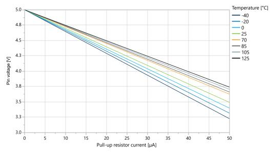
Figure 33-33. I/O Pin Pull-Up Resistor Current vs. Input Voltage (V<sub>DD</sub> = 5.0V)
