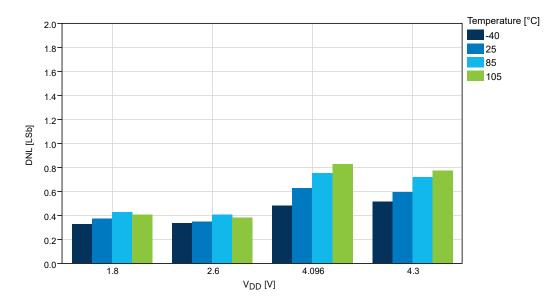
Figure 33-57. DNL vs. V<sub>REF</sub> (V<sub>DD</sub> = 5.0V, f<sub>ADC</sub> = 115 ksps, REFSEL = External Reference)
