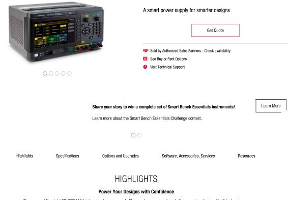
The compact Keysight EDU36311A triple-output power supply fits anywhere on your bench. You can view its sizeable 7-inch color display and monitor all outputs simultaneously from any angle. Each output is independent — connect your outputs in series for higher voltage, in parallel for additional current, or stack them to provide 0 to ±30 V. A sequencing feature enables and disables outputs in a set pattern to power up control logic before powering the rest of your design.
