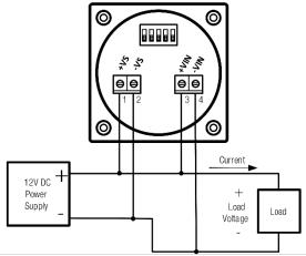
It is also possible to use the meter to monitor voltage in a circuit that is independent of the meter's power supply circuit, as shown in the schematic below. When used in this way, the meter's current measuring terminals may electrically float with respect to its power supply terminals, as long as the voltage difference between the two terminal pairs remains within +/- 48V of each other.
