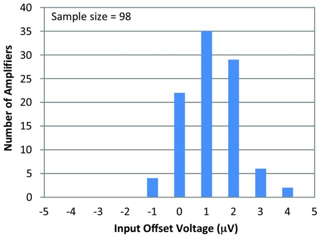
Figure 1. Input Offset Voltage Distribution with 3.3 V Supply
