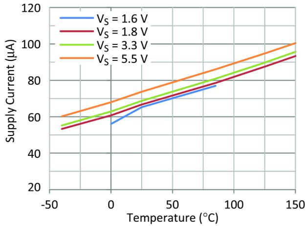
Figure 27. Quiescent Current Per Channel vs. Temperature
