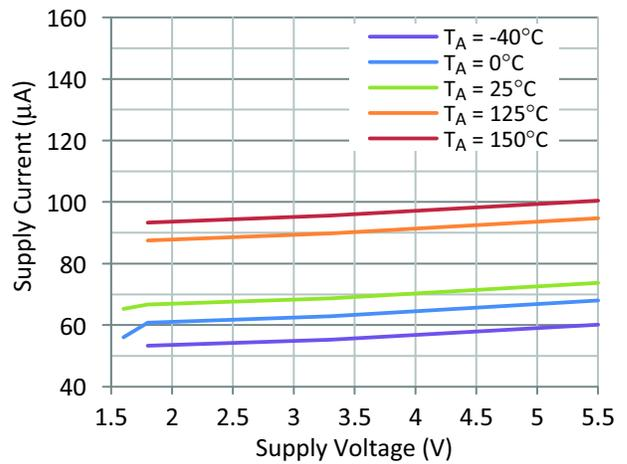
Figure 28. Quiescent Current Per Channel vs. Supply Voltage
