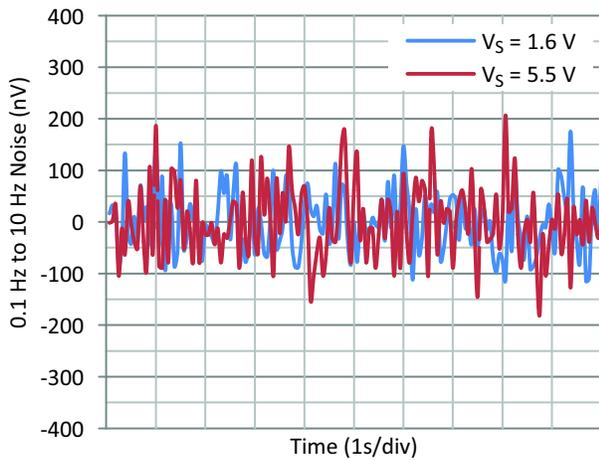
**Figure 19. 0.1 Hz to 10 Hz Noise**
