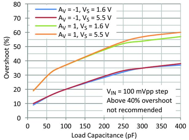
**Figure 24. Small Signal Overshoot vs. Load Capacitance**
