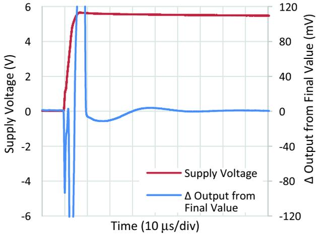
Figure 33. Power Up Time with 5.5 V Supply
