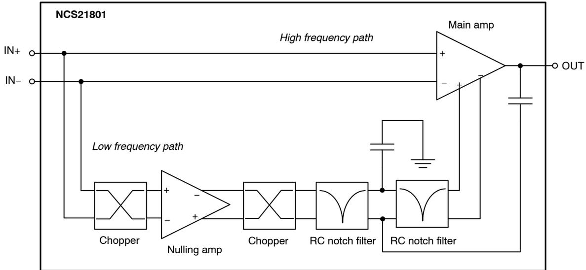
Figure 38. Simplified Schematic of the Chopper-stabilized Amplifier Architecture
