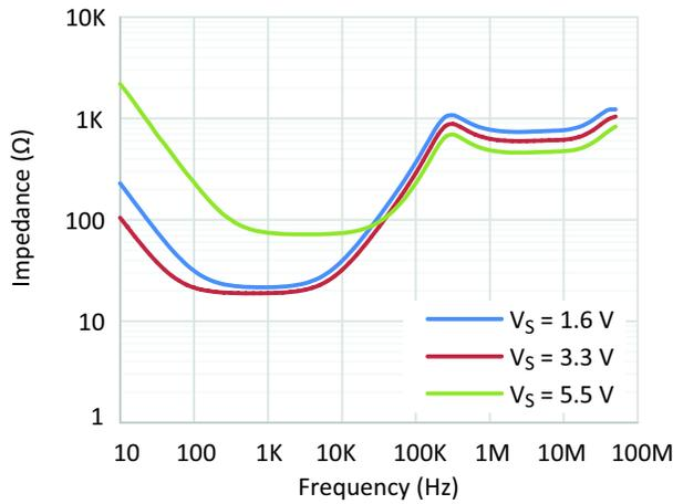
**Figure 23. Open Loop Output Impedance vs. Frequency**
