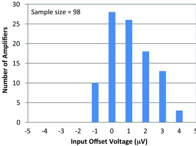
Figure 3. Input Offset Voltage Distribution with 1.6 V Supply
