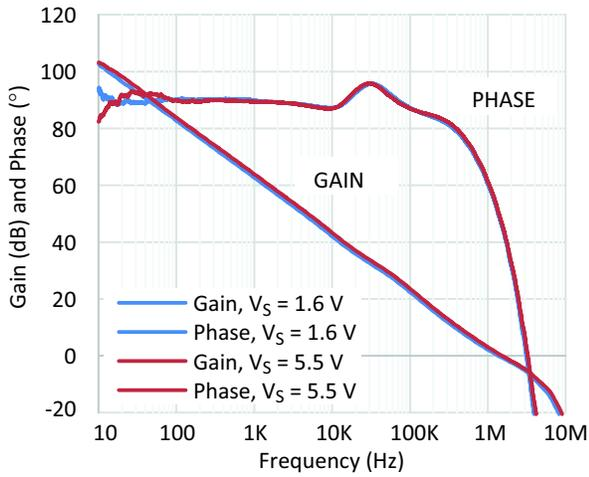
Figure 9. Open Loop Gain and Phase vs. Frequency
