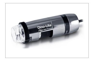
The AM7115MZTL is part of the Long Working Distance (LWD) range and with its Long Working Distance and magnification range from 10 – 140x, it is suitable for a wide range of applications where extra distance to the object or a larger field of view is required. The extra working distance and larger field of view make this model an ideal solution for tasks such as repair, rework or assembly or for working with bulky or fragile objects that cannot be touched.
