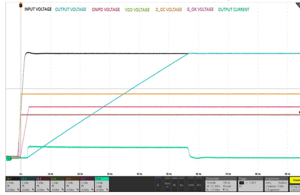
Figure 28. Startup by ON/PD (no load)
