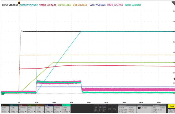
Figure 26. Startup by V_{IN} ( C_{OUT} = 6200\ \mu\text{F} , no load)
