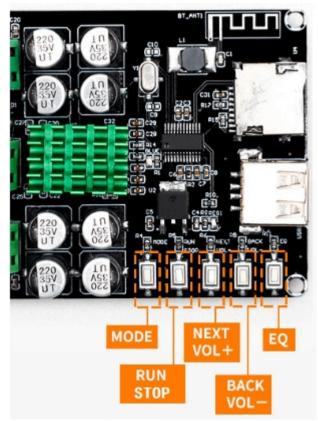
MODE: switch mode. When there is no TF-card or U-disk plugged in, the module enters Bluetooth Mode by default. The mode can be switched when plugging in SD-card or U-disk.
