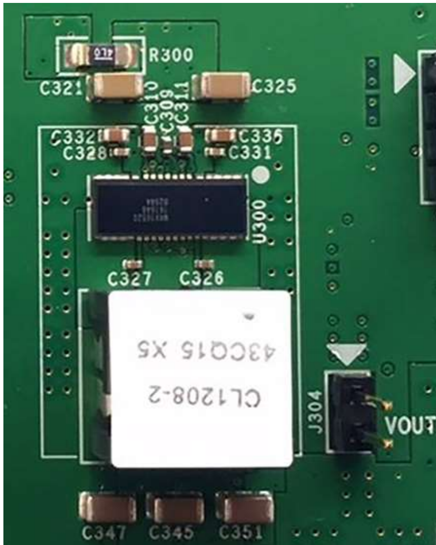
Figure 5. 60A two-phase coupled inductor buck converter PCB.
