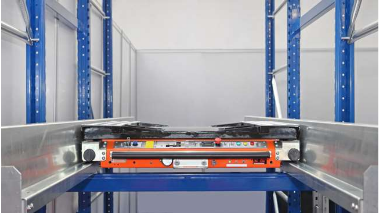
Figure 1. Warehouse automated pallet shuttle.
