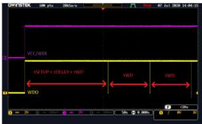
Figure 6. MAX6369 with SET0 = V_{\text{CC}} , SET1 = V_{\text{CC}} , and SET2 = V_{\text{CC}} .
