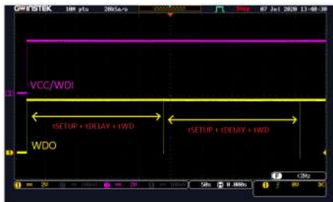
Figure 7. MAX6369 with SET0 = V_{\text{CC}} , SET1 = WDO, and SET2 = V_{\text{CC}} .
