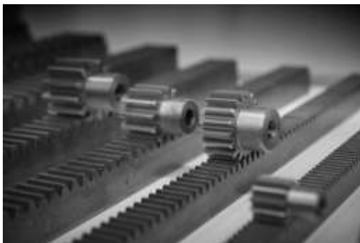
Figure 1. A diagonal view of metal pinion gears on toothed bars with high-precision linear toothed wheels.
