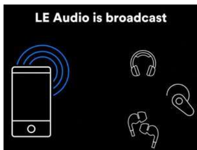
Figure 3. LE Audio can broadcast to unlimited sink devices.
