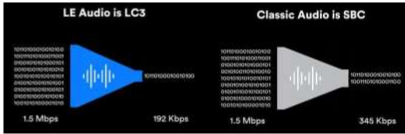
Figure 4. LC3 improves the codec efficiency.
