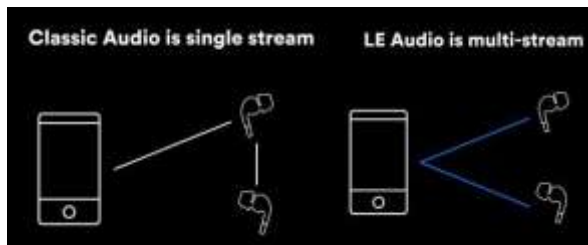
Figure 2. LE Audio adds support for multiple streams.
