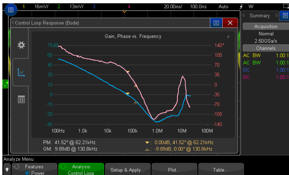
Figure 3. Control loop response test using the DSOX3054PWR Power Better Bundle.
