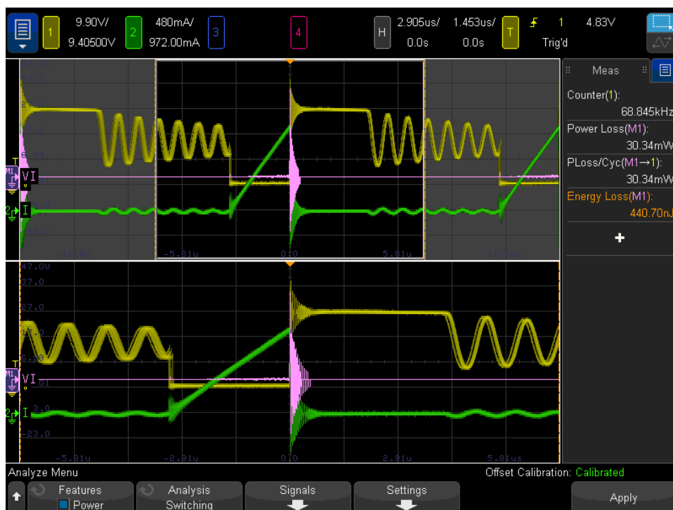
Figure 4. Switching loss measurement using the MSOX4154PWR Power Best Bundle.
