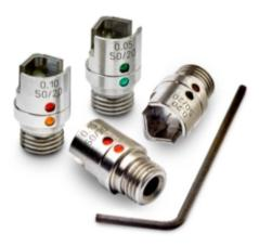
The slit evaluation kit includes four different slit diameters integrated in the SMA 905 connectors. With a hexagon socket screw key, you can easily switch the SMA connector with the integrated slit and adjust the optical performance to your application. A smaller slit leads to higher optical resolution but decreases the spectral sensitivity of the device. Changing from a 20  $\mu$ m diameter to a 50  $\mu$ m slit doubles your optical throughput and allows detecting weaker signals.
