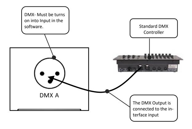
One DMX Output must be turns on into an input in the Options windows. To access this window click on the software menu: Tools > Options. Then click to select the device section as following:
