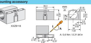
Recommended to use for sensor applications at operating temperatures -25 ... 0 °C (-13...32 °F)
