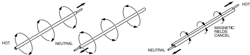
To avoid the canceling effect of the opposing magnetic fields and optimize the transmitted signal, the conductor to be traced should be separated from the return conductor by utilizing a remote return path.
