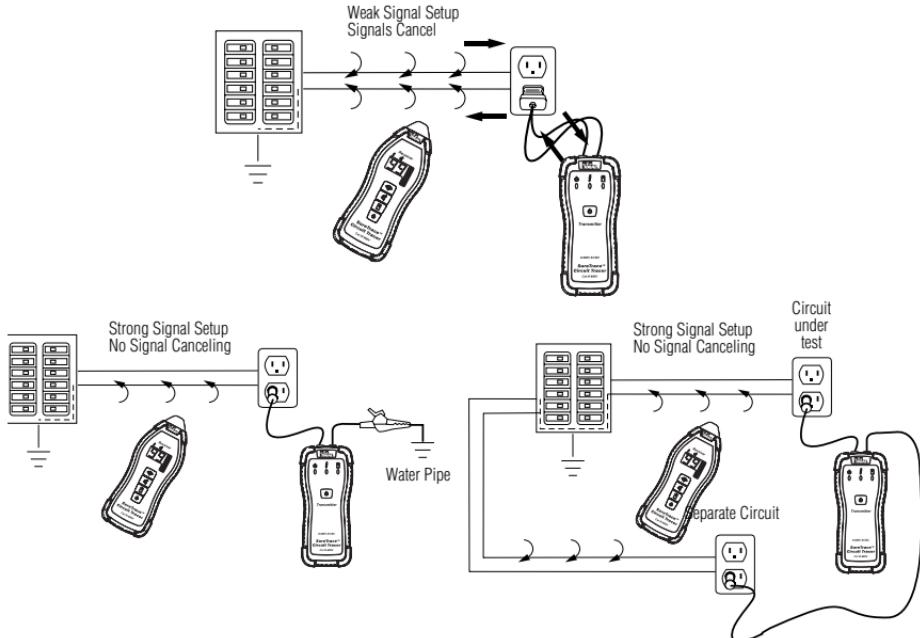
If unsure that the remote return path chosen is a good one, use a multimeter to measure the resistance between the circuit neutral and the remote return path. If  $>100\Omega$ , a different return path should be selected.
