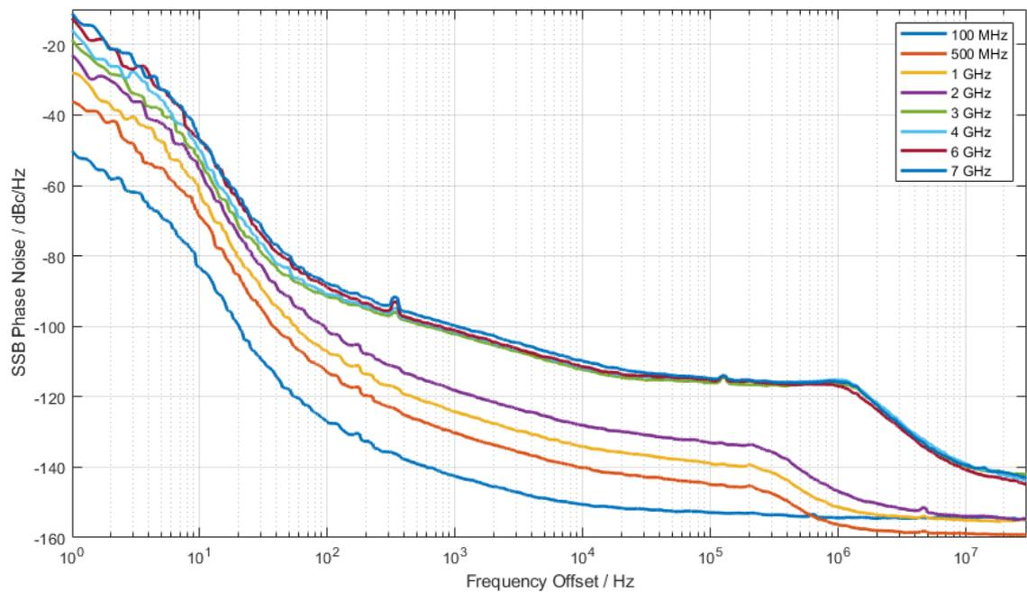
Measured SSB phase noise for different carrier frequencies, with R&S<sup>®</sup>SMCVB-K709 option
