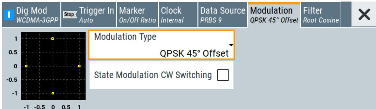
Figure 6-4: Display of the used modulation type
