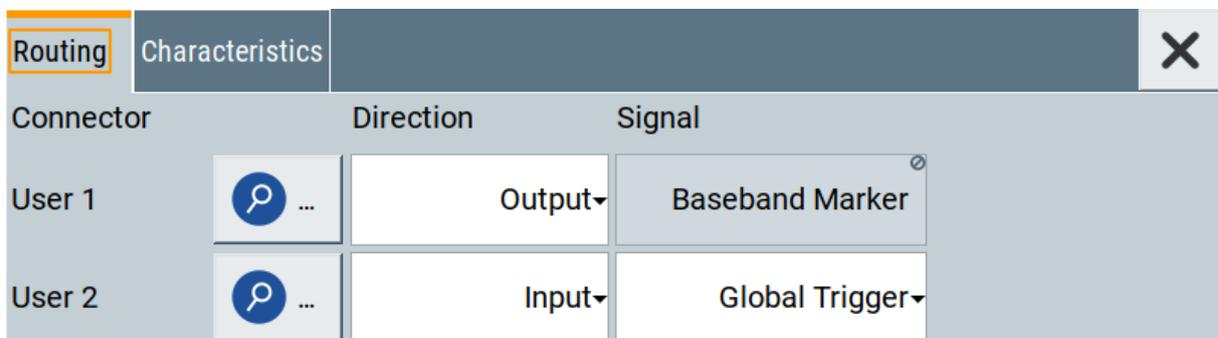
**Figure 6-5: Signal mapping to the global connectors**
