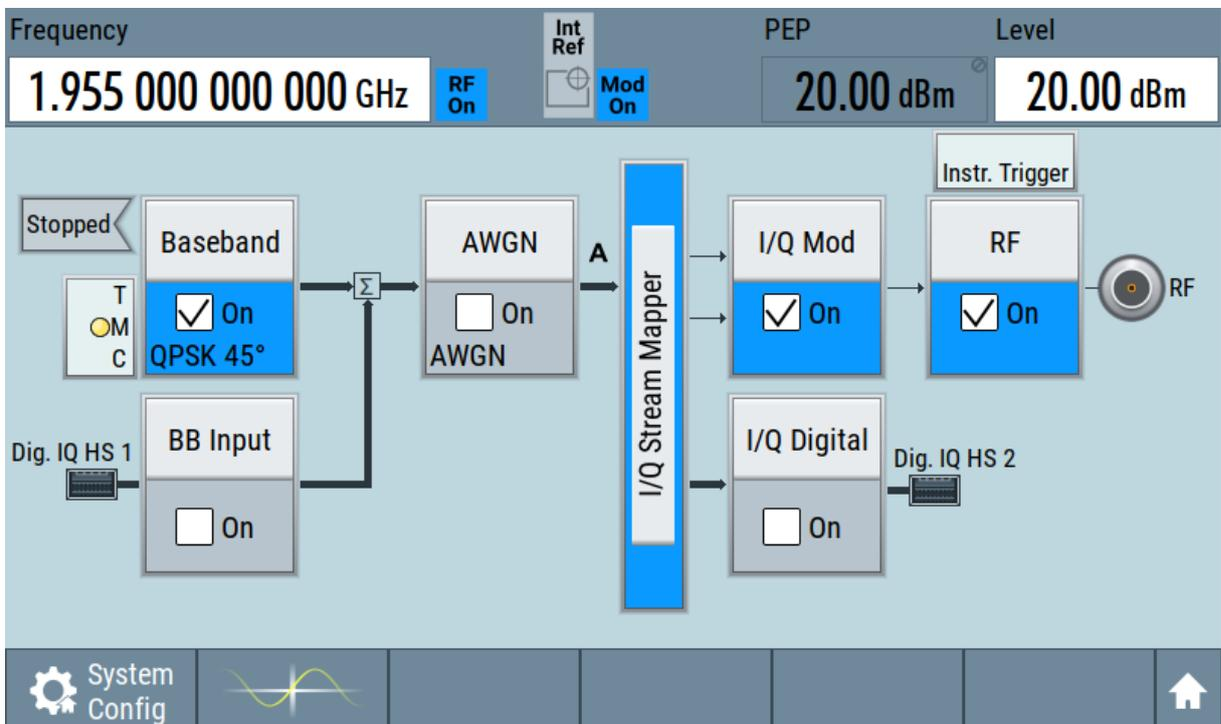
Figure 6-3: Block diagram: Generating a digitally modulated signal
