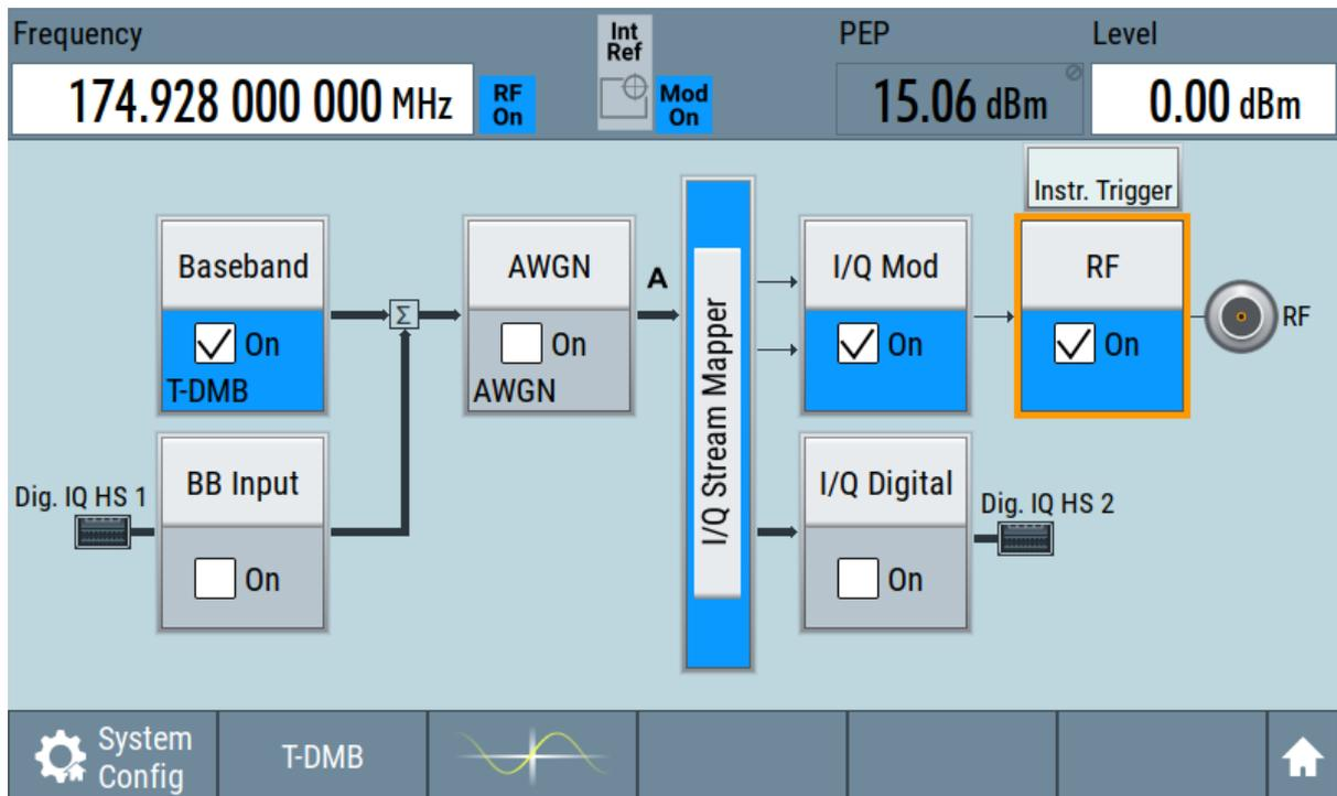
The instrument generates a DAB test signal with the set frequency, and level.
