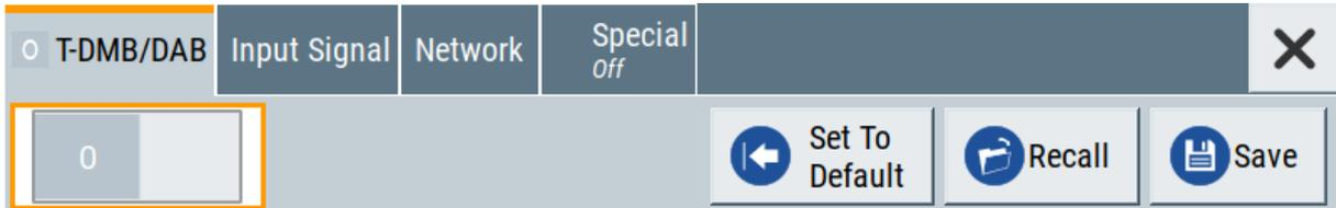
As in the user interfaces of all broadcast standards, the "T-DMB/DAB" dialog is divided into several tabs. The "T-DMB/DAB" tab comprises the primary settings of the standard.
