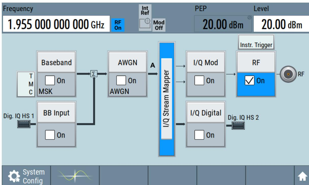
Figure 6-1: Block diagram: Generating an unmodulated signal
