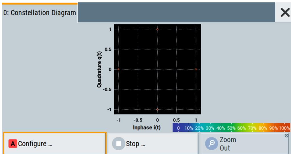
The "Constellation Diagram" displays the 3GPP FDD signal.
