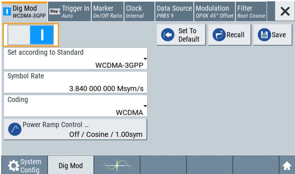
The instrument activates automatically "I/Q Mod", uses the internal trigger and clock signals, and generates a WCDMA-3GPP signal, modulated with a QPSK 45° offset modulation.
