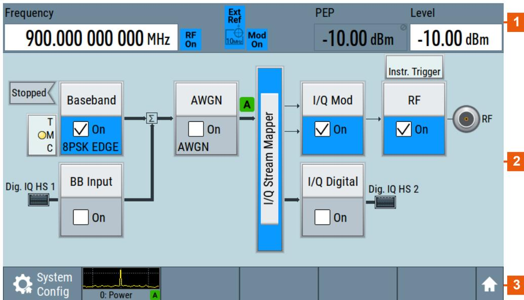
Figure 8-1: Block diagram
