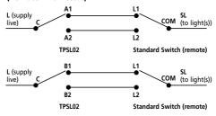
Either standard switch could be a TPSL01 or half a TPSL02). Connections to SL (lights) and L (supply live) can be swapped if required.
