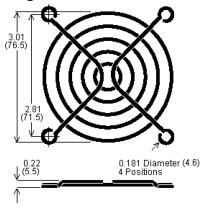
Newark.com/multicomp-pro Farnell.com/multicomp-pro Element14.com/multicomp-pro Dimensions : Inches (Millimetres)
