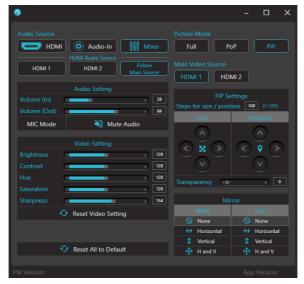
Audio Source: Switch the audio source type to record between embedded HDMI audio, analogue line input, or the audio mixer.
