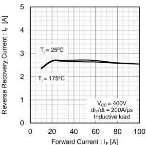
Fig.24 Typical Diode Rrverse Recovery Charge vs. Forward Current
