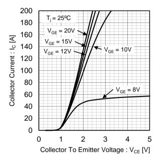
Fig.6 Typical Output Characteristics
