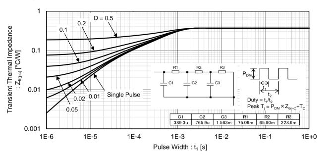
Fig.28 Typical Diode Transient Thermal Impedance
