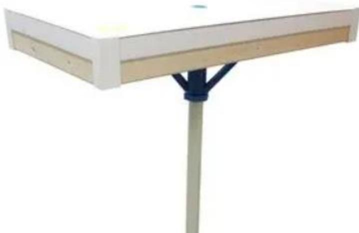
Heavy duty turn table for MegIQ radiation measurement system
