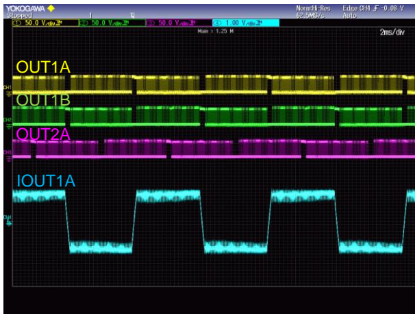
Figure 14. FULL STEP ( CLK : 600 Hz )
