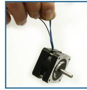
**Do not** hold motor by lead wires.
