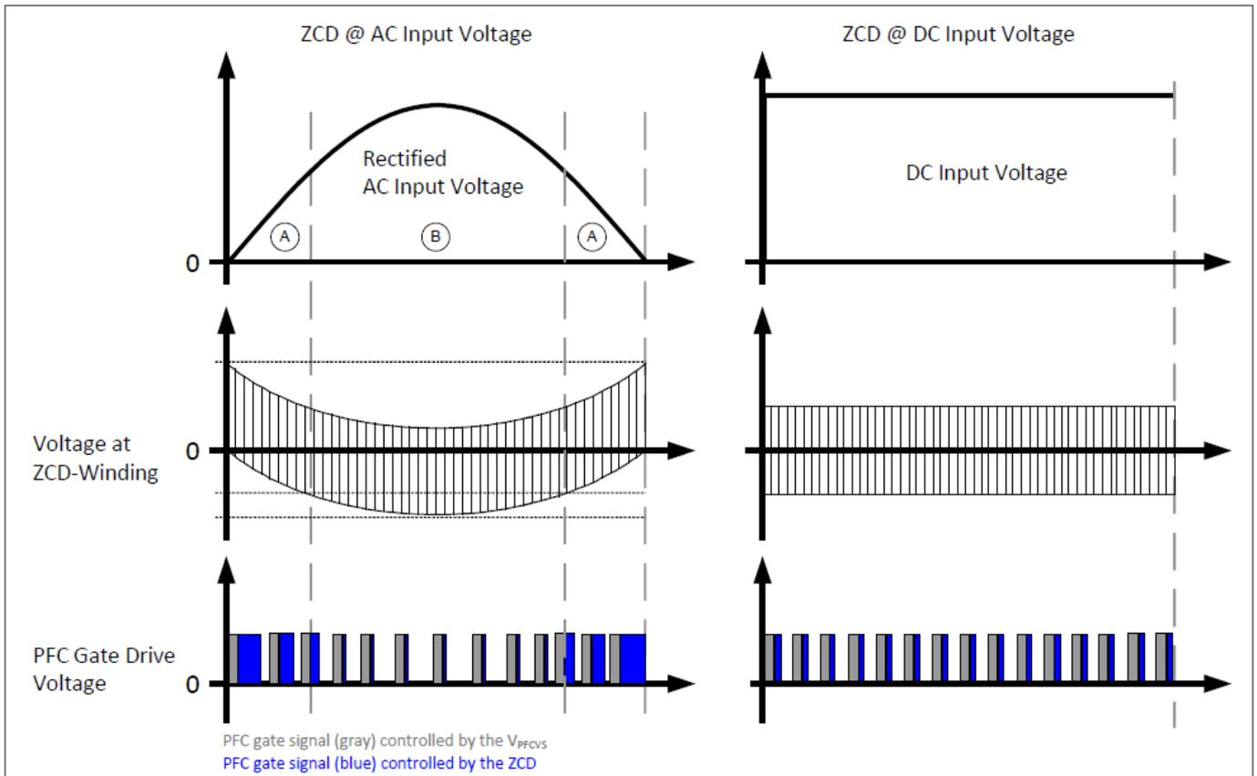
**Figure 14** THD improvement – automatic pulse width extension
