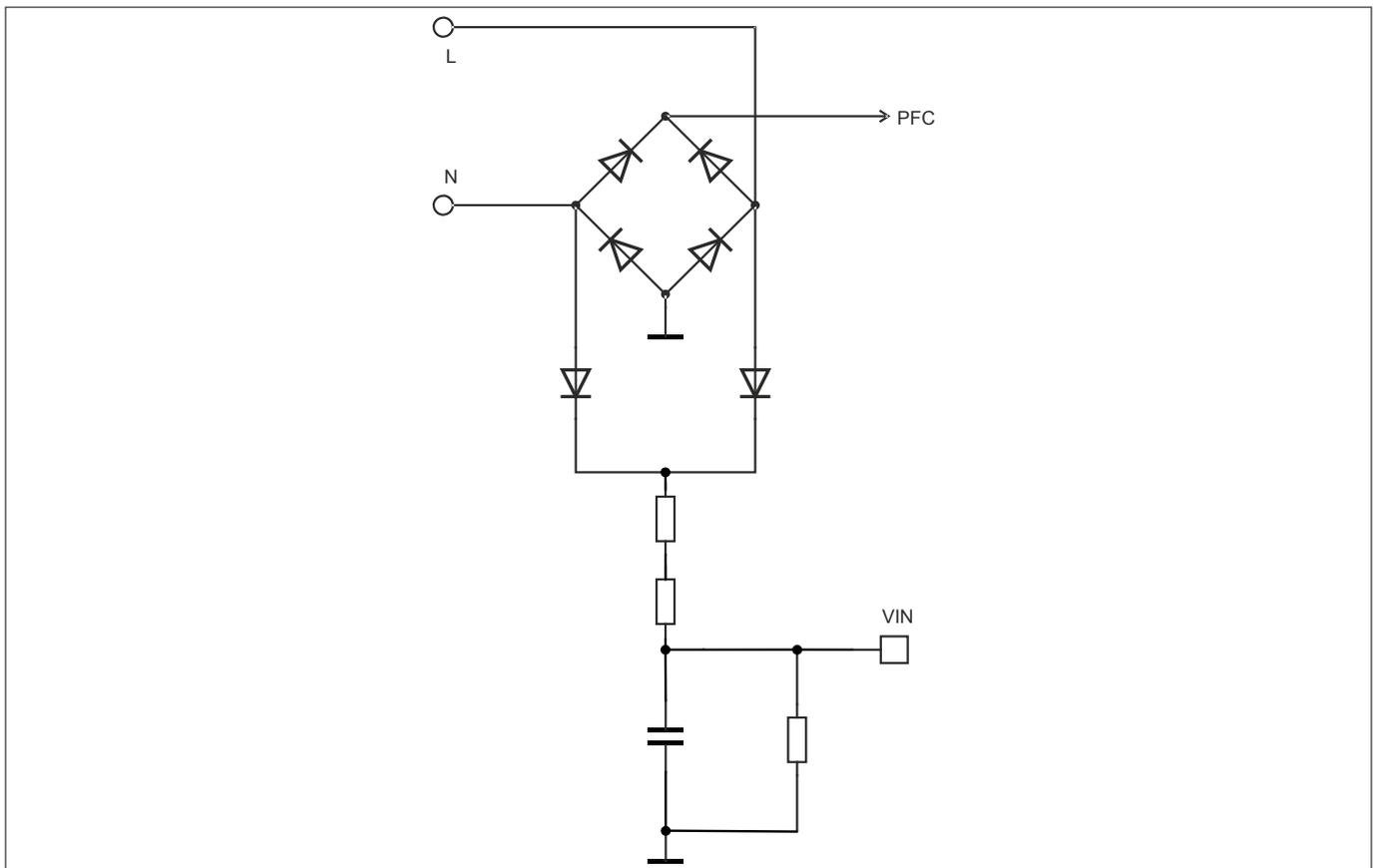
Figure 11  $V_{IN}$  pin circuit
