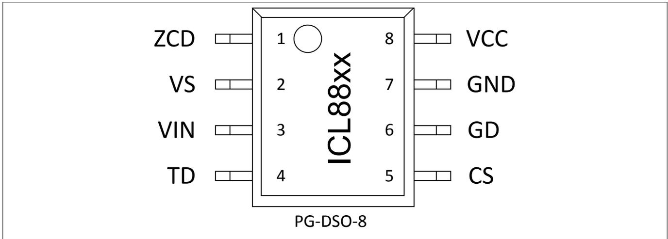
Figure 3 Pin configuration
