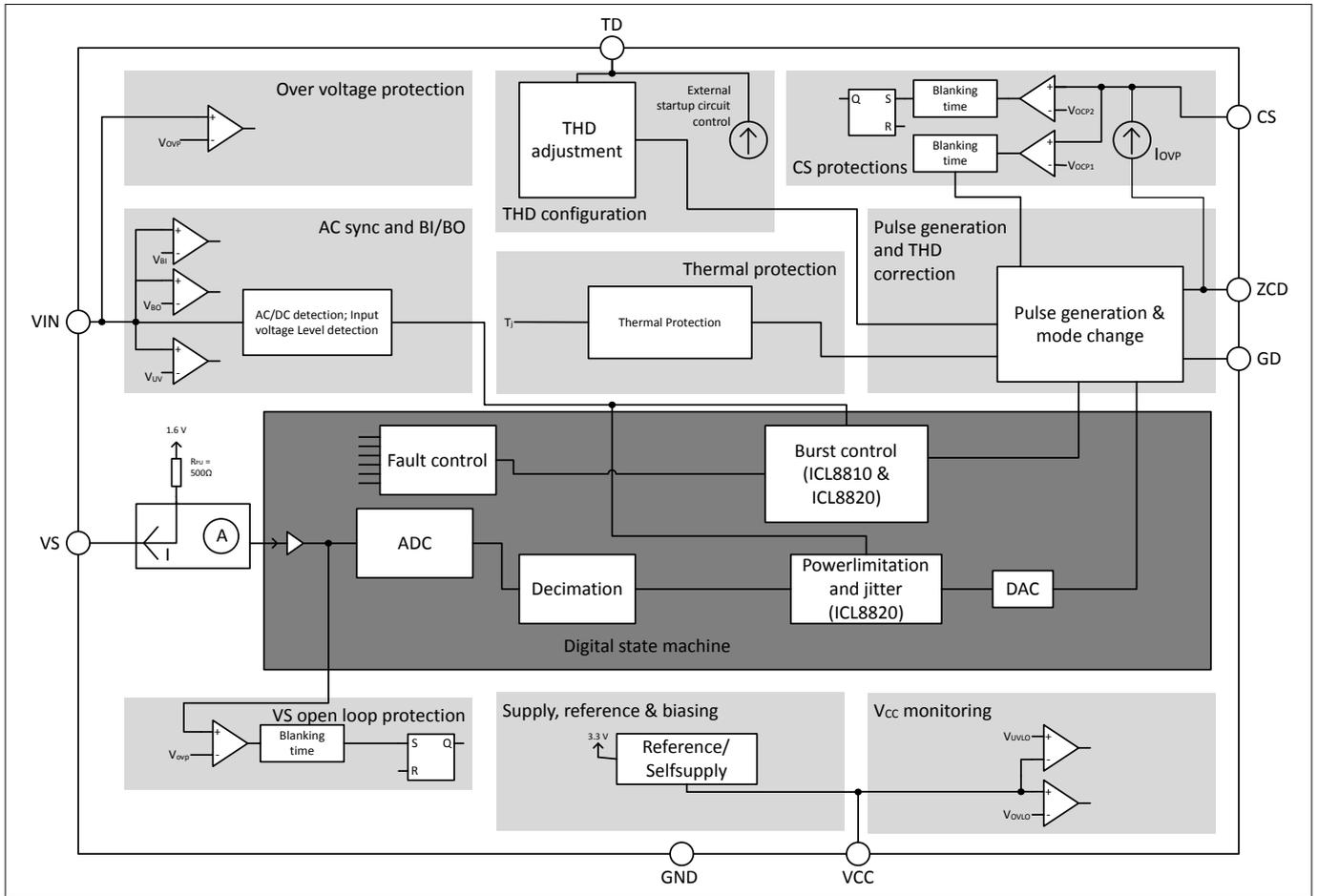
Figure 4 Block diagram
