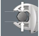
The parallel smooth jaws of the Joker 6004 allow surface pressure and can thus prevent rounding of the bolt or screw head, which can occur during power transmission on corners.
