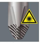
A precisely-focused laser creates a sharp-edged surface structure. This laser treatment results in an edge hardness of up to 1000 HV 0.3. Wera Lasertip "bites" itself into the screw head and prevents any slips out of the recess. It is available for screwdrivers for slotted, Phillips and Pozidriv screws.
