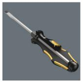
Wera makes its Kraftform handles from several materials with different properties. The core is made from a hardwearing plastic that holds the blade securely even when subjected to great forces. The yellow soft zones of the external mantle consist of a softer material with more friction resistance for high torque transfer. The black areas with a harder surface prevent the hand from sticking to the handle enabling you to adjust your grip more quickly.
