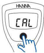
From measurement mode, press and hold the ON/OFF button until "CAL" is displayed.
