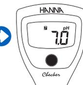
Meter will exit to measurement mode and the calibration tag will be displayed.
