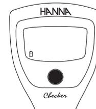
The Checker® features a low battery indicator. When the battery is running low, the tag will blink on screen. When the battery has been depleted, "Erb" will appear on screen and the meter will turn off.
