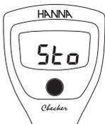
When the reading is stable, the stability indicator will disappear. "Sto" will be displayed when the calibration is saved.
