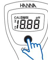
Press the ON/OFF button to turn the meter on. All tags will be displayed.
