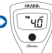
If using pH 4.01 or pH 10.01 as a second point, continue two-point procedure at right.
