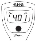
If pH 4.01 or pH 10.01 buffer solution is used as the first point the value of the buffer is recognized and displayed with the blinking stability indicator.
