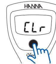
Place meter in calibration mode. Press and hold ON/OFF until "CLr" is displayed. The meter will now be at default calibration. No tags will be shown in measurement mode until calibration is performed.
