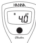
Meter will exit to measurement mode and the calibration tag will be displayed.
