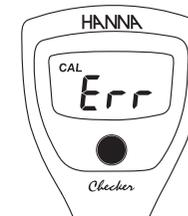
In calibration mode, if the meter displays an "Err" message when in the correct fresh buffer solution then the probe should be cleaned. Place the probe in the HI700601 cleaning solution for 15 minutes. Rinse with purified water and place in storage solution for 1 hour before calibrating. If the "Err" message persists then the HI1271 probe should be replaced.
