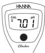
If pH 7.01 buffer solution is used as the first point the buffer is recognized with the blinking stability indicator.
