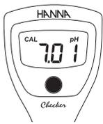
When "7.01" blinks on the display, place the tip of the probe into a pH 4.01, 7.01, or 10.01 buffer solution.
