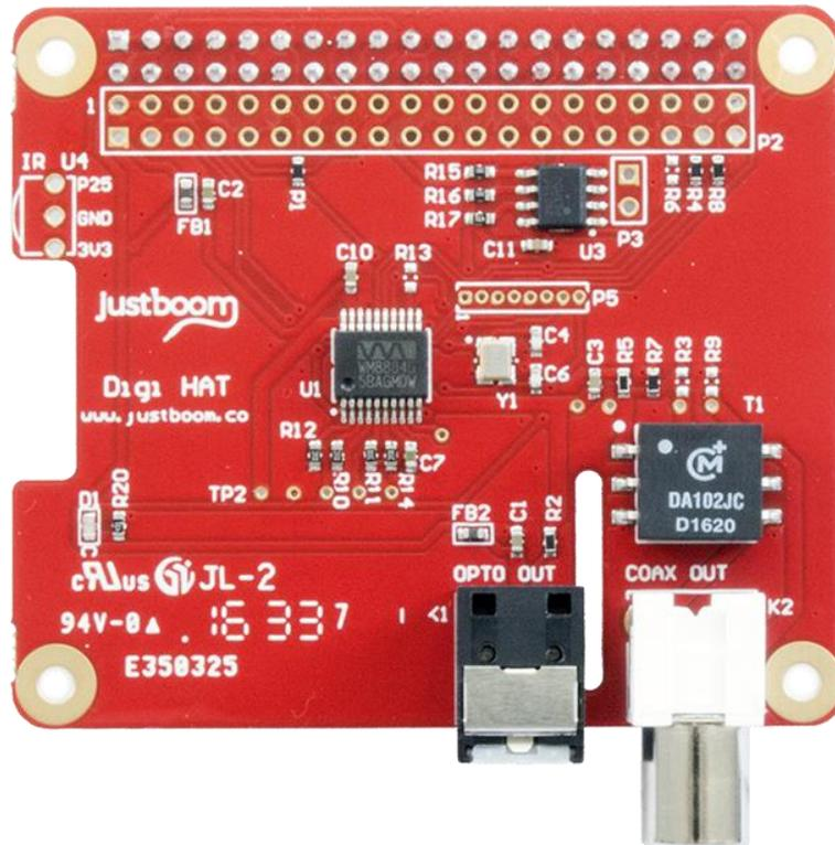
The JustBoom Digi HAT is a high resolution digital audio output add on board for the Raspberry Pi. Simply stack the plug-and-play add on board (HAT) onto your Raspberry Pi A+, B+, 2B, 3B, 4B and it will be ready to use immediately. The JustBoom Digi HAT produces an unmodified, high quality, digital audio data stream for bit-perfect transmission to your hifi system.
