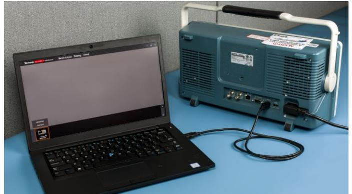
The instrument connected to a computer through the USB interface
