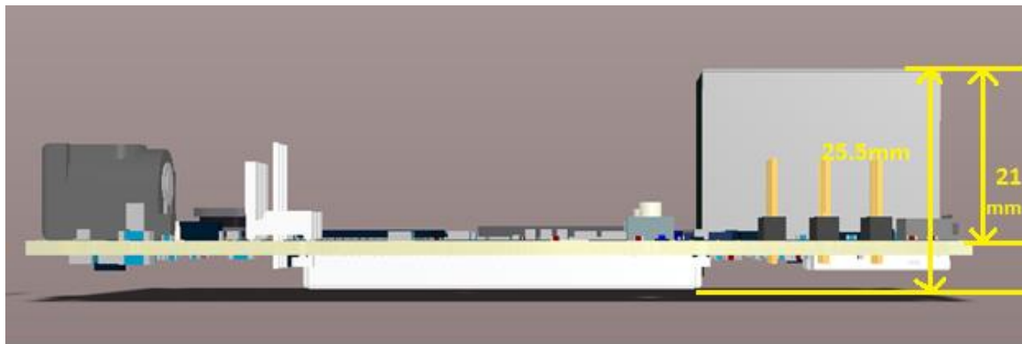
Figure 19 – MicroZed Side Vertical Dimensions
