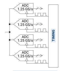
**PARALLEL** Simultaneous sampling in 12-bit mode and up to 1.25 GS/s sampling rate.
