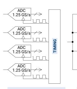
**4-CHANNEL** Up to 10-bit resolution and 1.25 GS/s sampling rate. TIME-INTERLEAVED Maximum 5 GS/s sampling rate on one channel in 8 or 10-bit mode.
