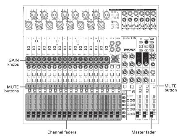
1. Use to adjust the input signals while inputting sound from instruments and mics.
