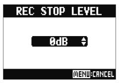
Recording will stop automatically when the level of the MASTER fader output stays below the set level for the amount of time set in step 2.
