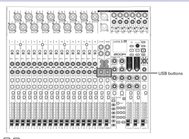
1. Turn USB 1-2 USB 3-4 ON for the stereo channel to use for input.
