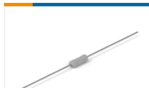
TE Part #9-1676123-2 1/2W SM M/OX 5% 5K1
