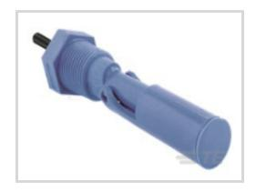
Liquid Level Switch Mounting: Side Entry Medium/Liquid: Alcohol, Fuel, Oil Contact Form: A Fitting: 1/2 NPT Liquid Level Switch Material: Glass Filled Nylon 6.6 All Horizontal Liquid Level Switches (20)
