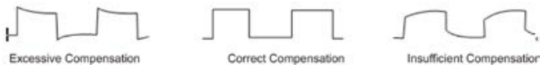
Picture 1-2 Probe compensation calibration
