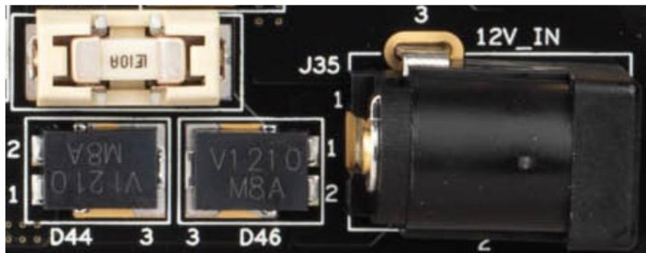
Figure 1.3. 12 V DC Power Supply
