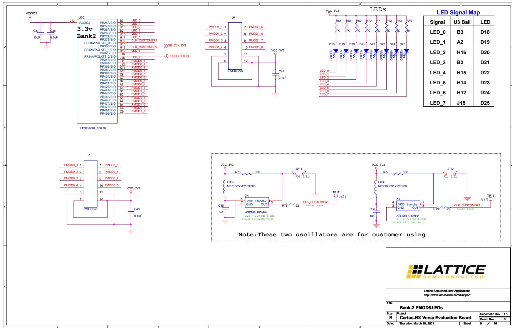
Figure A.6. Bank-2 PMOD&amp;LEDs
