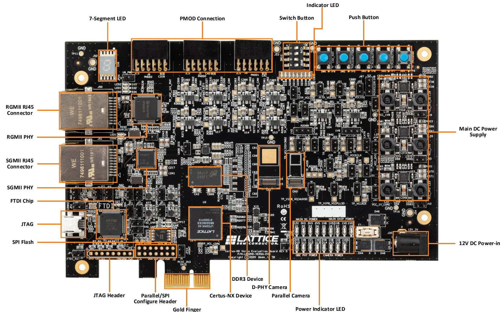
Figure 1.1. Top View of Certus-NX Versa Evaluation Board
