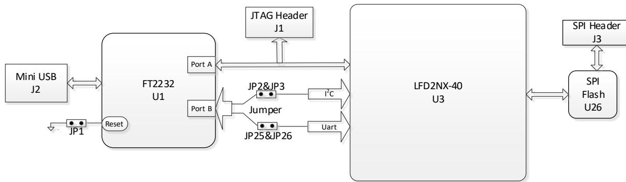
**Figure 4.1. Configuration and I<sup>2</sup>C Architecture**
