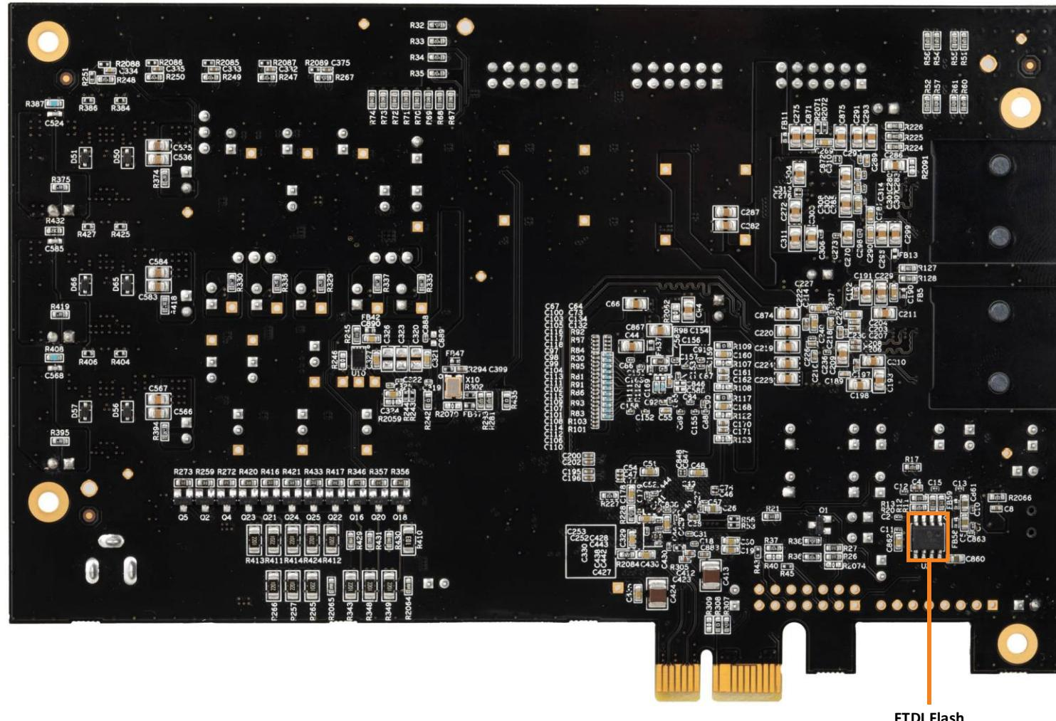
Figure 1.2. Bottom View of Certus-NX Versa Evaluation Board
