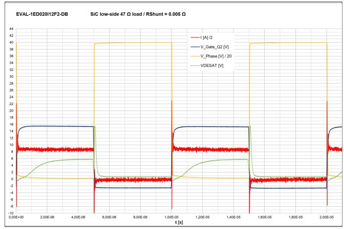
Figure 15 Switching resistive load according to figure 7
