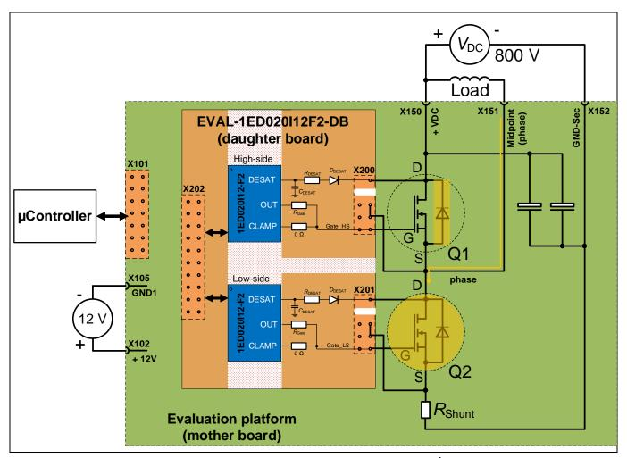
Figure 7 Motherboard equipped wit daughterboard and SiC MOSFET's for low-side measurements
