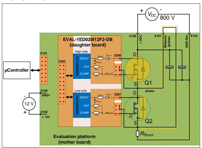
Figure 17 External circuit for high-side measurements
