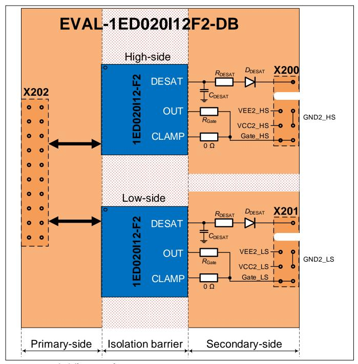
Figure 5 Blockdiagramm of EVAL-1ED020I12F2-DB
