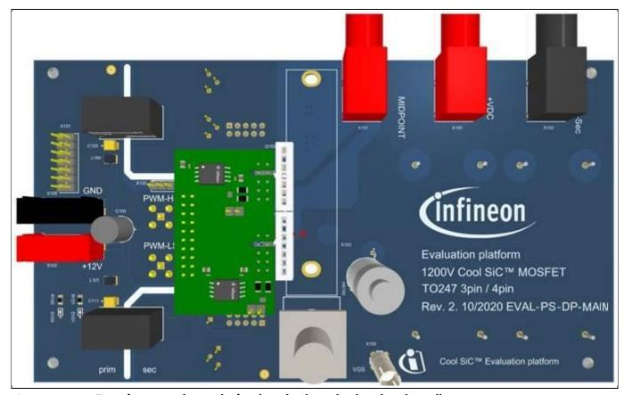
Figure 3 Top view complete solution (motherboard + daughterboard)
