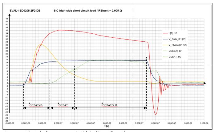
Figure 18 Short ciruit measurement at high-side configuration
