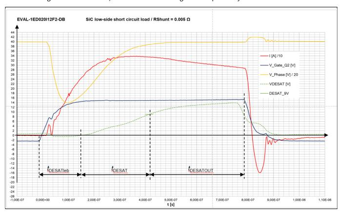
Figure 16 Short ciruit measurement at low-side configuration
