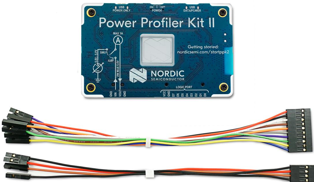
Figure 1: PPK2 board and cables
